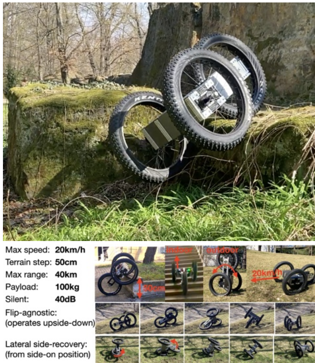
Fig. 1. Helhest R&D platform: Outline of dynamic capabilities, lateral and longitudinal side-recovery.
