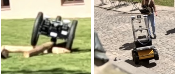
Fig. 3. Experimental environment and platforms: Left Helhest on wooden obstacles; Right Husky on stairs.
