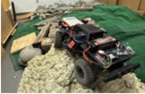
Fig. 5: Unseen Test Environments with Rocks/Boulders, Wooden Planks, Astro-Turf, and Expanding Foam.
