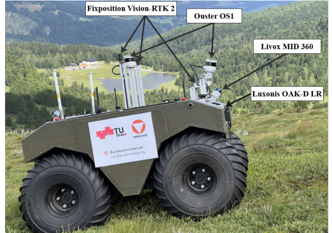
Fig. 1. Warthog and its sensor setup shown on the mountain in the Seetaler Alps.
