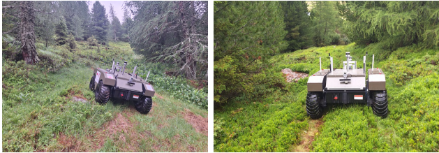
Fig. 5. Example conditions on Route 2 of the autonomous navigation evaluation. The challenges of this route include the steep incline leading up the mountain, the overhanging branches, and the vegetation on the path.
