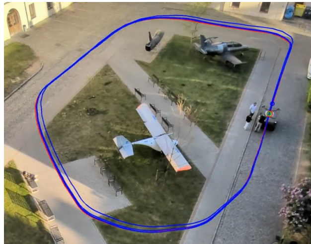
Fig. 7: Repeated traversals using the BearNav method. The red curve represents the recorded route, while the blue curves correspond to the reconstructed traversals.
